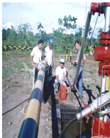
Photograph 4. Repsol Crude Oil Sampling
