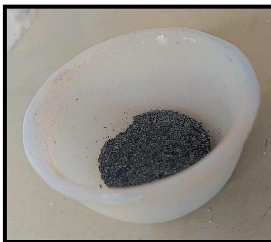
Fig 12.1 determination of ash value of betel leaf
