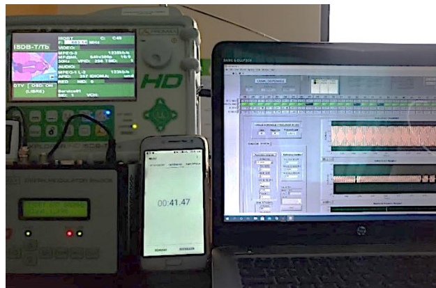
Figure 26. System response time for the critical case
